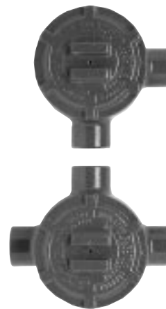
Junction boxes are U.L., CSA and FM approved for explosion proofing in Class I, Division 1, Groups B, C, D, E, F, G
